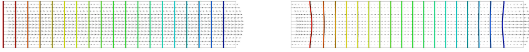
Figure 3.7: Channel flow with stable finite elements (left) and with the stabilized form (right). Along with the velocity vectors, the pressure isolines are illustrated.
